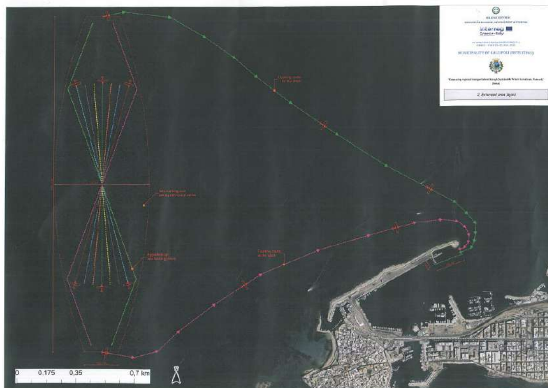
Figure 9 - Spatial Planning Analysis of the water aerodrome in the port of Gallipoli
